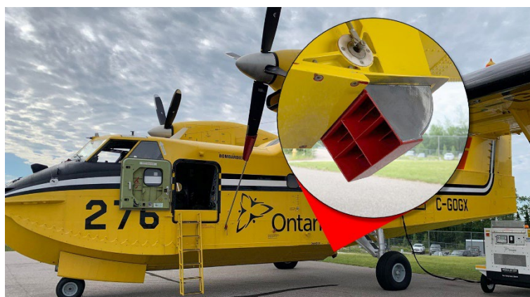
The CL-415 fills its water tanks in a matter of seconds by extending these small ports on the bottom of the plane while skimming across the water.
